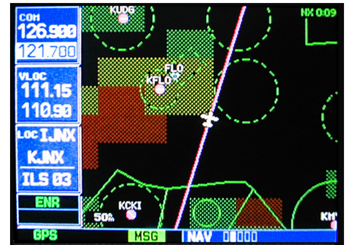
GNS 530 Datalink Screen shot of same weather. Notice the large blocky presentation of weather due to the lower resolution (36 sq. mi.), which might cause you to deviate much more than needed.
